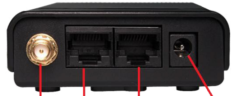
WAN Port LAN Port Power Jack 12V DC-In Antenna Connector
